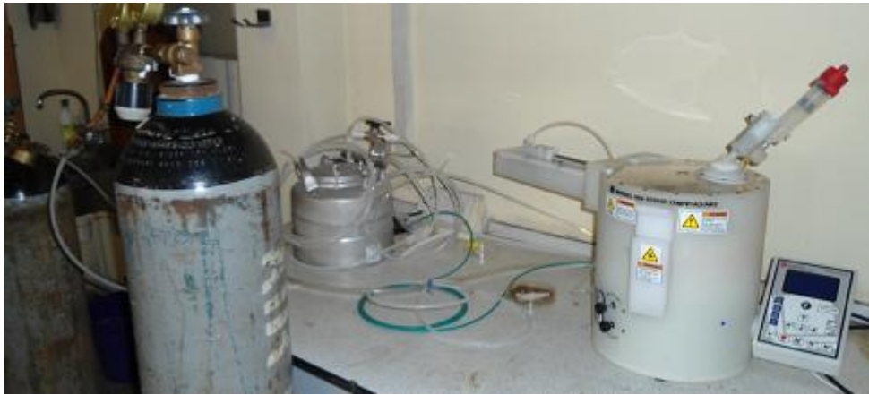
Figure 13.4: The Spin Coater
