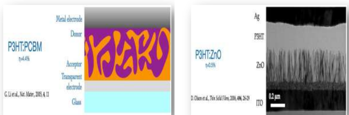
Figure 2.30: Active layer polymer blends in Bulk Heterojunction solar cell structure. [Adapted from NREL]
