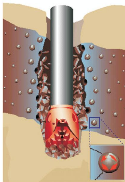
Figure 2.10: Drilling through Induced Over-Pressured Shale (Adapted from [12])
