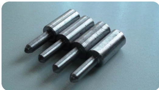
Figure 3-4 a & b: Pins machined from the pickaxes (left); Disc made of steel for wear experiment (right) at SCC Pipe Yard, Abuja – Nigeria.
