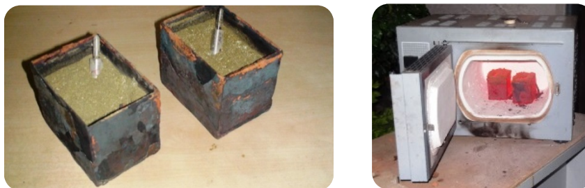
Figure 3-5 a & b: Steel pins in the pulverized cyanide pack and heat-treated.
