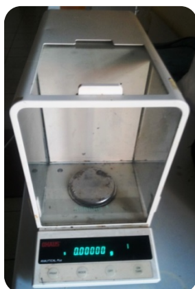
Figure 3-10: Electronic weighing balance with 10^{-5} sensitiveness at Sheda Science Complex, SHETSCO – Abuja.
