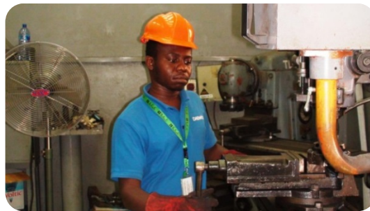
Figure 3-3: Using the milling machine to prepare samples at SCC Pipe Yard, Abuja – Nigeria.
