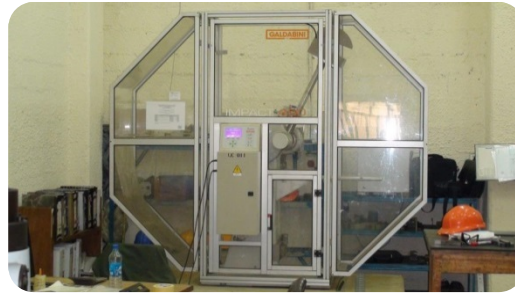
Figure 3-8: Charpy impact equipment at SCC Pipe Yard, Abuja – Nigeria.
