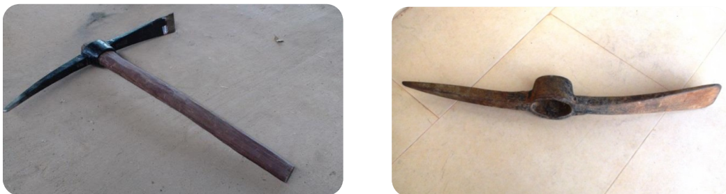
Figure 3-1 a & b: New “Champion” pickax (left) and the metal head of a used “Champion” pickax (right) used for analysis in this research.
