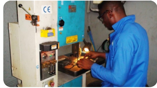
Figure 3-2 a & b: Cutting and shaping samples using an anvil device, electric saw and hammer (left); and using a band saw (right) at SCC Pipe Yard, Abuja – Nigeria.
