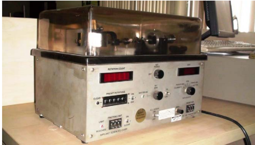
Figure 2-5: A pin-on-disc tribometer at AUST, Abuja – Nigeria.
