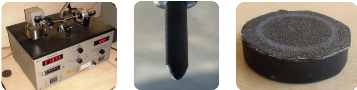
Figure 3-9a, b & c: Wearing of pin on SiC grit paper.
