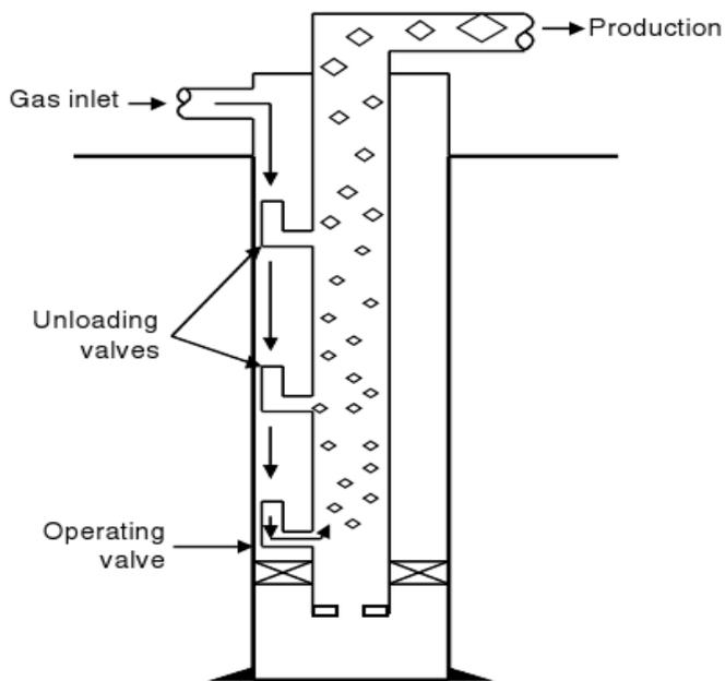
**Figure 2.6:** Configuration of a typical gas lift well
