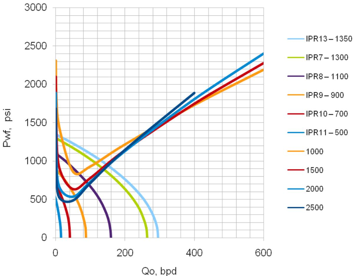
**Figure 4.10:** Performance of 1.5" tubing under varying GORs
