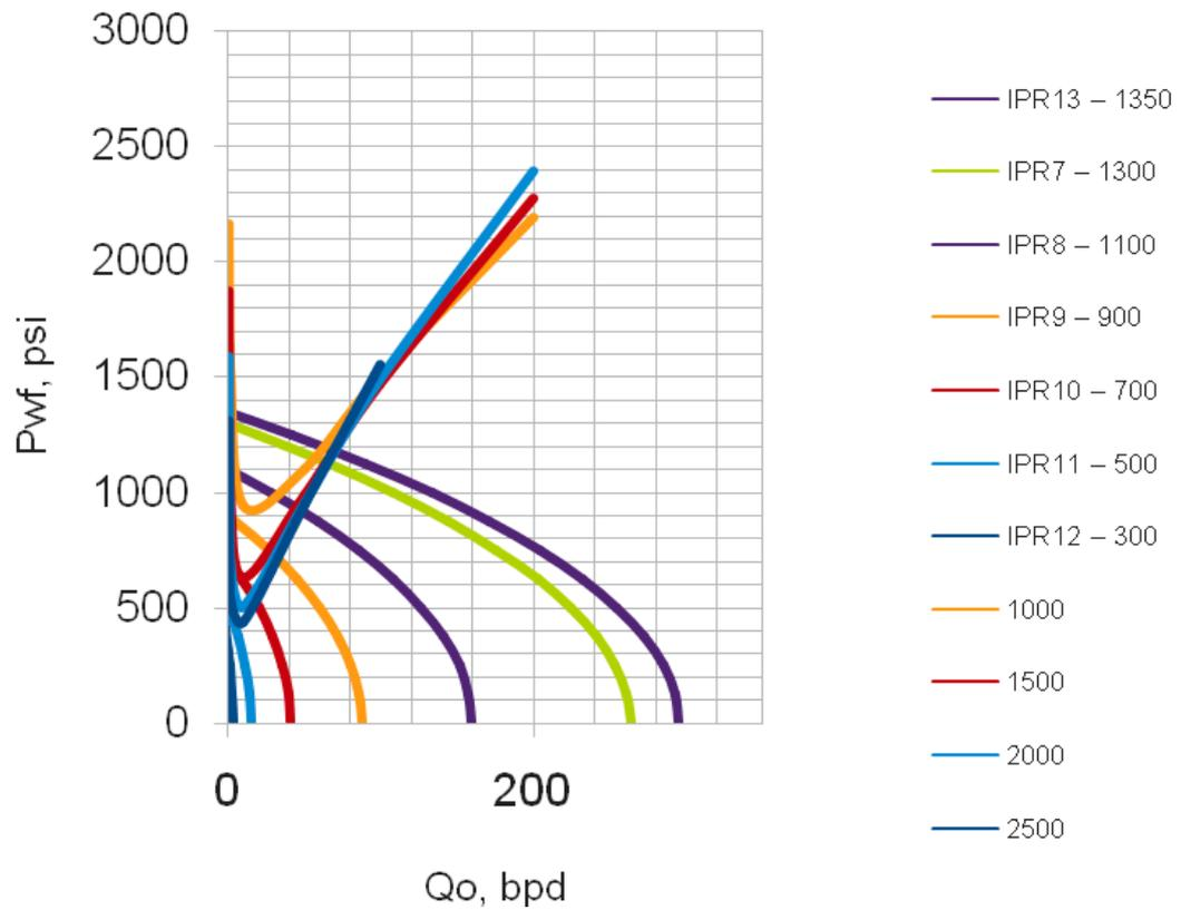
**Figure 4.11:** Performance of 1" tubing under varying GORs
