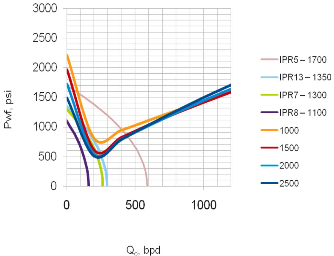
**Figure 4.9:** Performance of 2 3/8" tubing with varying GORs
