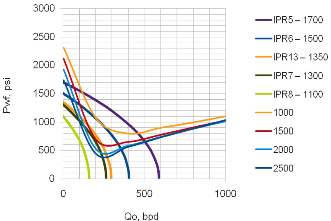
**Figure 4.8:** Performance of 2 7/8" tubing with varying GORs
