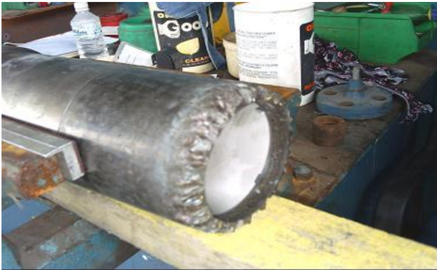
Fig 2.2: Eroded piston head (Source: Han et al., 2011)
