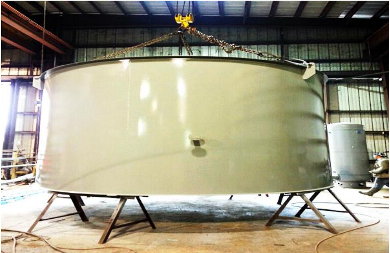
Figure 1.2: Large welded API-grade storage tank (Cembell Industries, 2017)
