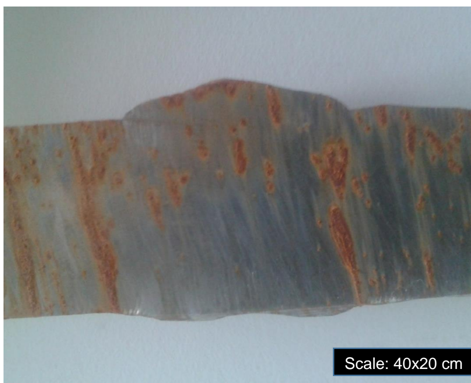
Figure 4.1: Corroded steel from the de-aerated methanol medium
