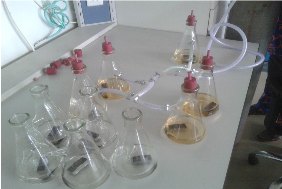
Figure 3.1: Experimental set-up showing methanol being purged with nitrogen
