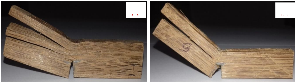
Figure 4.2: SENB samples after fracture toughness experiment (a) Arrester orientation (b) Divider Orientation
