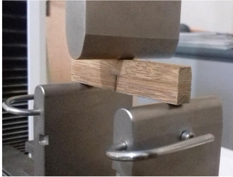
Figure 3.7: Test Setup and Loading of SENB Samples
