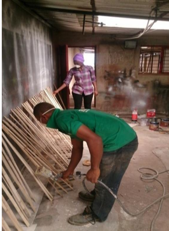
Figure 3.3: Spraying of Bamboo Strips
