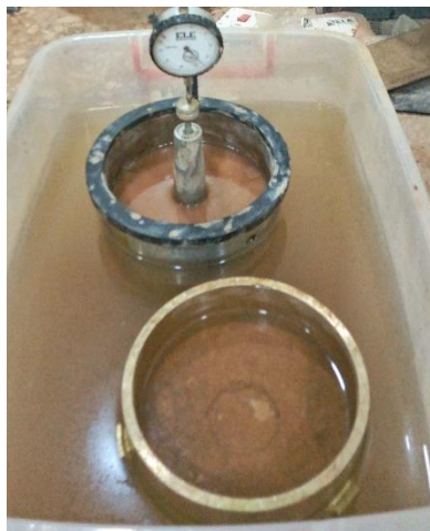
Figure 3. 15: Modified 1-D swell test set-up.
