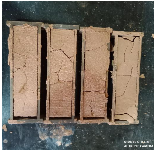
Figure 3. 17: Linear shrinkage bar test setup
