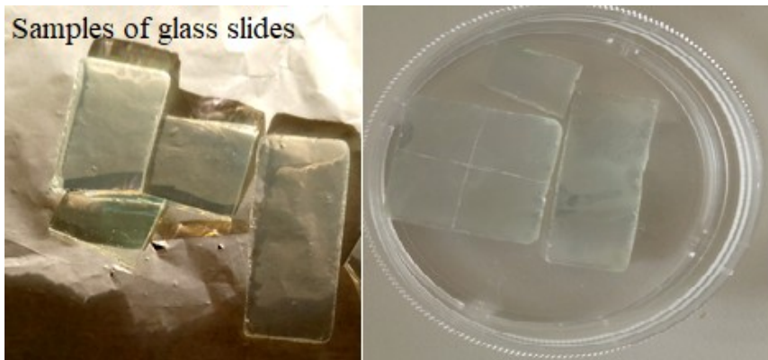
Figure 15: Samples of glass cut using diamond tip
