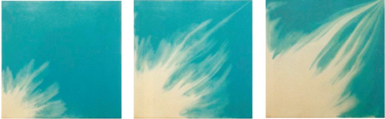
Figure 2.6: Schematic of Viscous Fingering (Source: perminc.com/resources).
