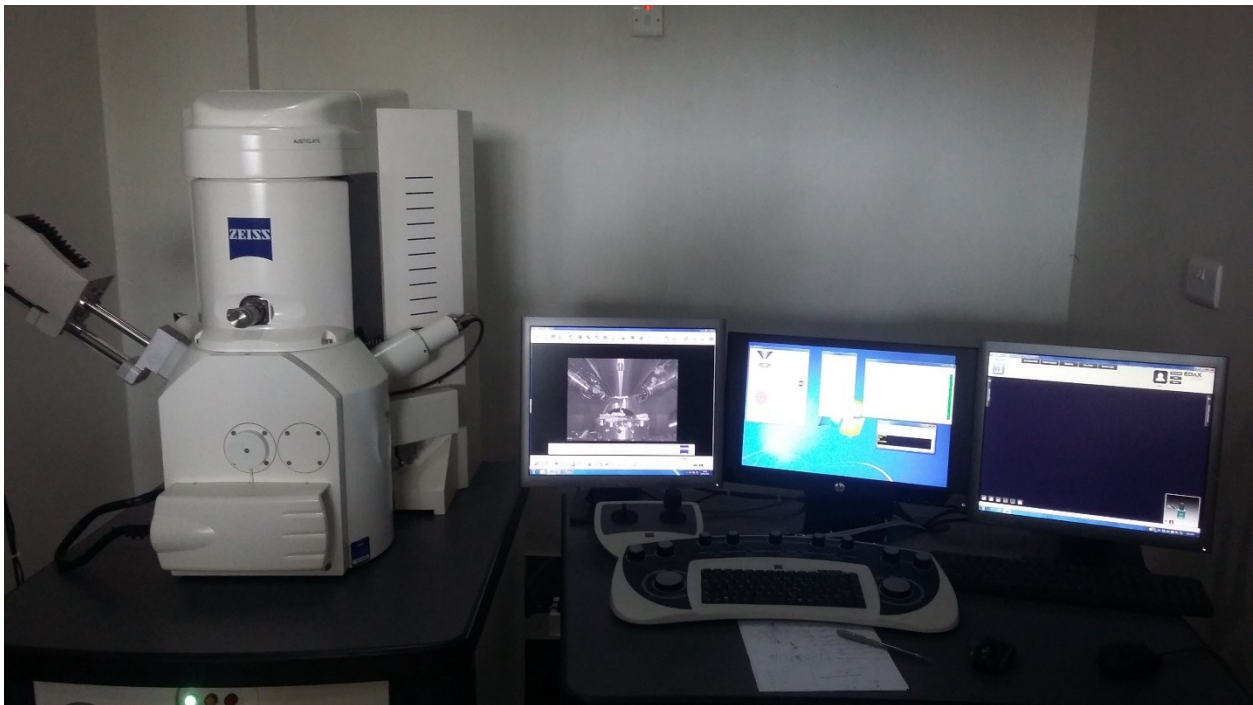
Fig. 3.2: Scanning Electron Microscope Instrument in EDX Mode
