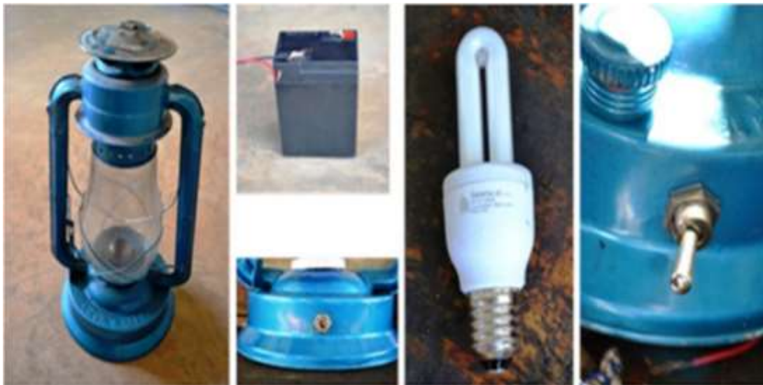
Figure 6.12: (Color online) Locally-purchased components, including a (a) hurricane kerosene lantern, (b) motorcycle battery, (c) compact fluorescent light-bulb, and (d) metal switch were collected and assembled. (e) The light-bulb, for example, was put into the place of the wick. (f) These modifications resulted in a converted solar-powered hurricane lantern.
