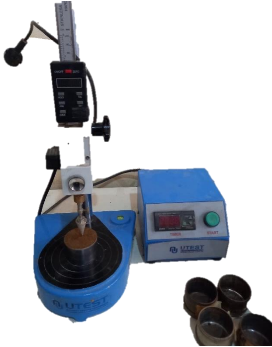
Figure 3.6. Liquid Limit with UTEST Cone Penetrometer and Moisture Cans
