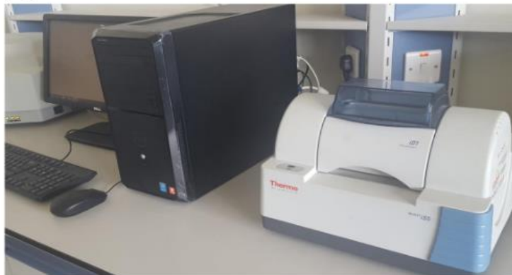
Figure 3.10. (g) Pellet placed in the sample holder of the FTIR instrument (h) FTIR Instrument setup
