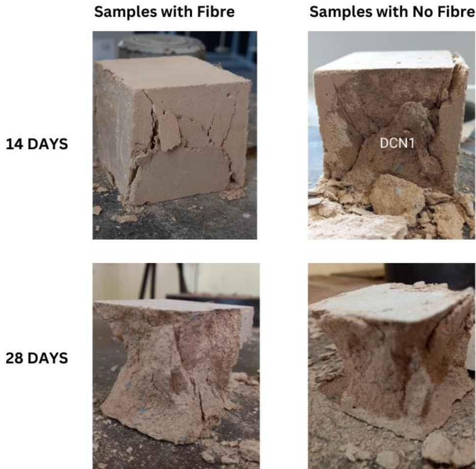
Figure 4.9b. Failure mode of samples at 14 days and 28 days compressive strength test.
