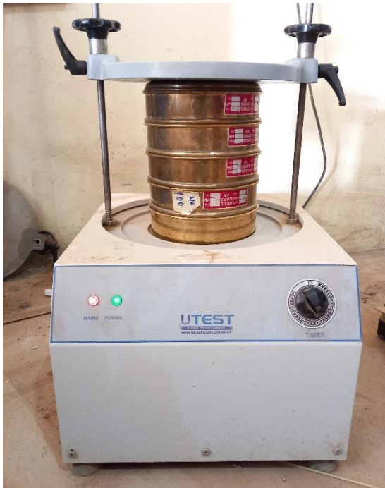
Figure 3.5. Sieve Analysis with UTEST Mechanical Sieve Shaker
