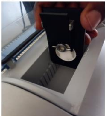
Figure 3.10. (g) Pellet placed in the sample holder of the FTIR instrument (h) FTIR Instrument setup
