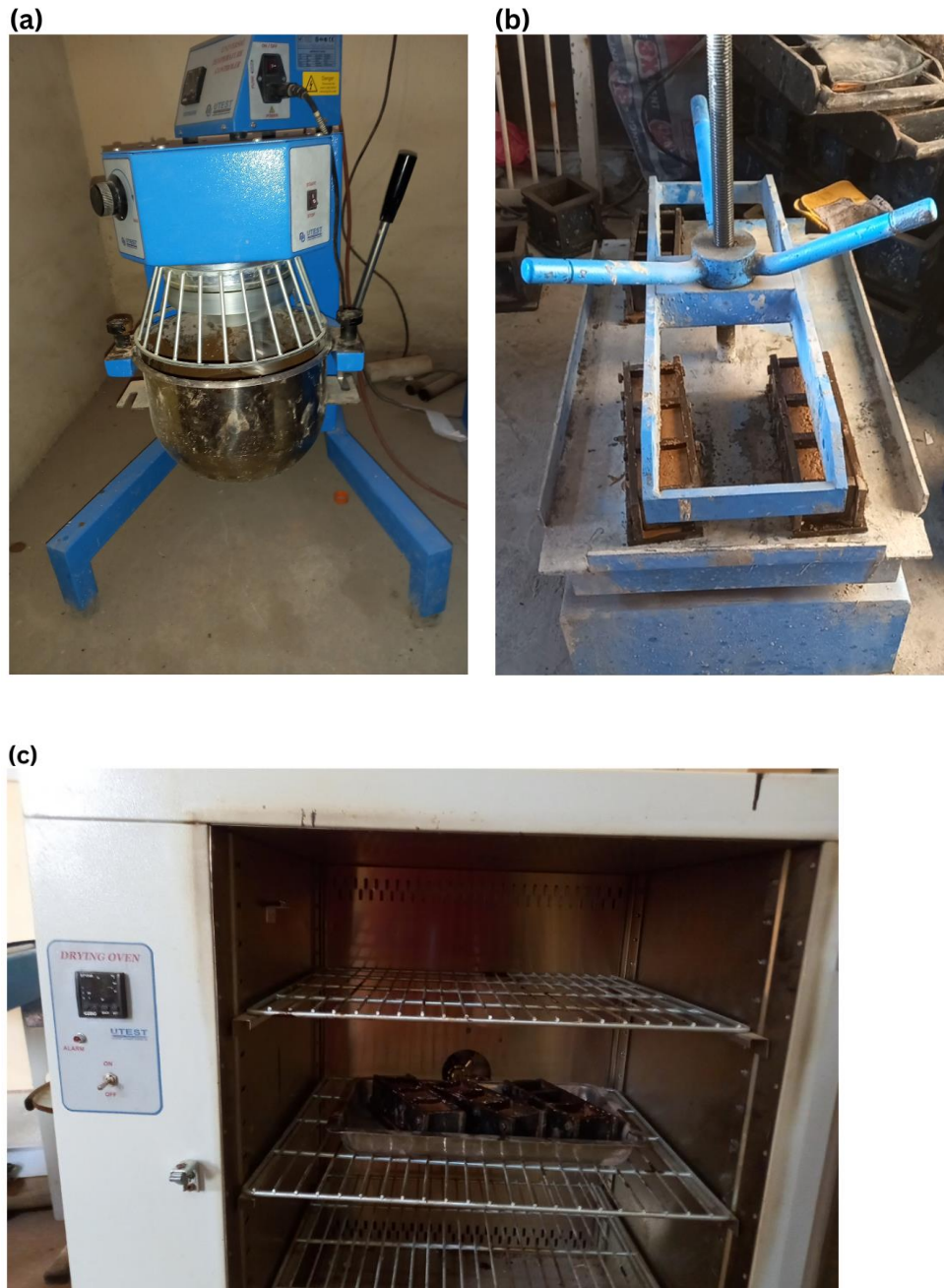
Figure 3.3. (a) Materials mixing with UTEST laboratory mixer (b) Vibrating samples with UTEST fixed amplitude vibrating tables (c) Drying samples with UTEST laboratory oven
