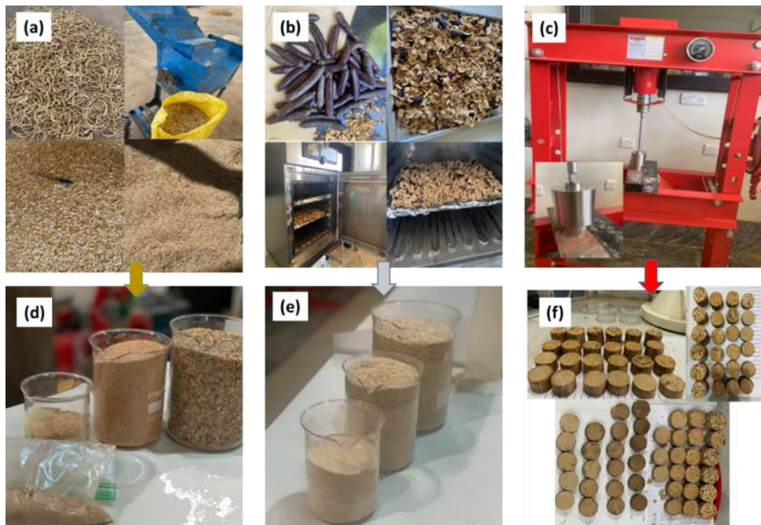
Fig. 23: Brikette-making process; (a) Biomass waste extraction of cowpea husks, (b) Biomass waste extraction of Prosopis africana pod, (c) Experiment molds and hydraulic press, (d) pulverized cowpea husks, (e) pulverized Prosopis africana pod, (f) the production of CPH-PAP-CSB brikettes
