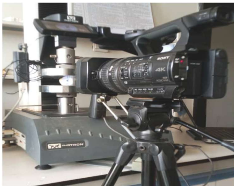
Fig. 2. The laboratory experimental setup for Brazil disc experiment for real-time imaging of the barite rock disc specimens.
