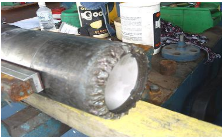
Figure 2.2: Eroded piston head (Source: Han et al., 2011)
