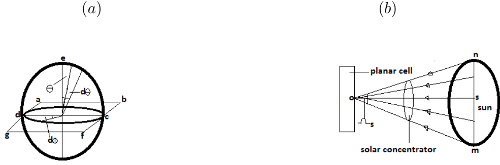
Figure 5.3: (a): a planar cell(abfg) emitting photons through the top surface. (b): a solar concentrator focuses sun rays on a planar cell.
