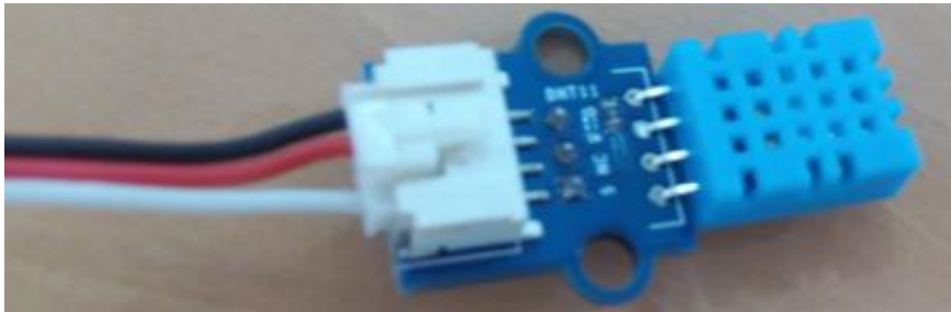
Figure 3.3: DHT11 Temperature-Humidity Sensor
