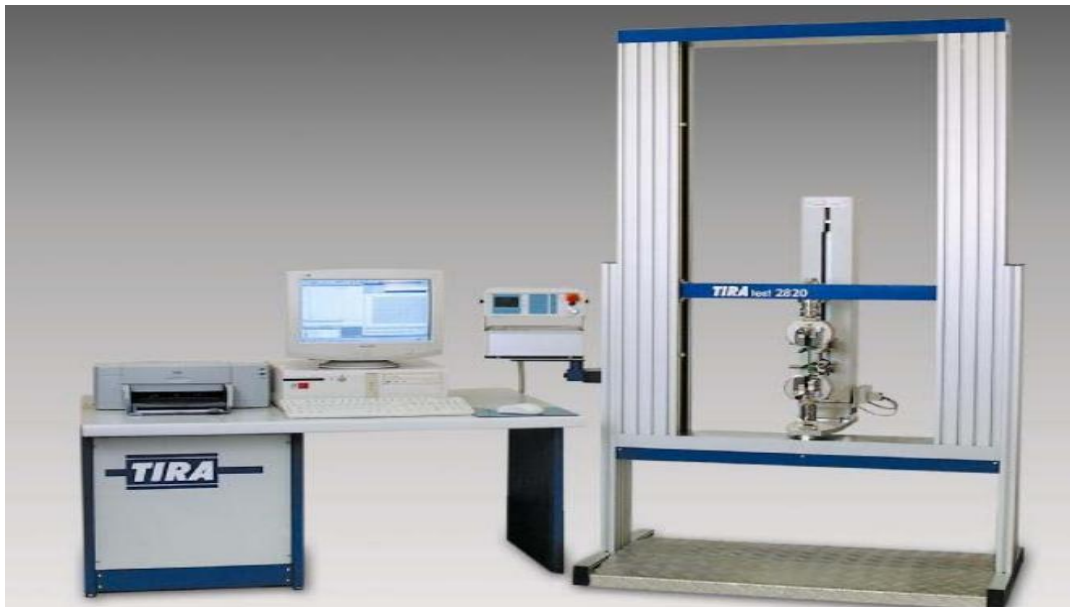
Fig. 3.02: Picture of Tiratest (Instron) model 2810 Universal testing machine.
