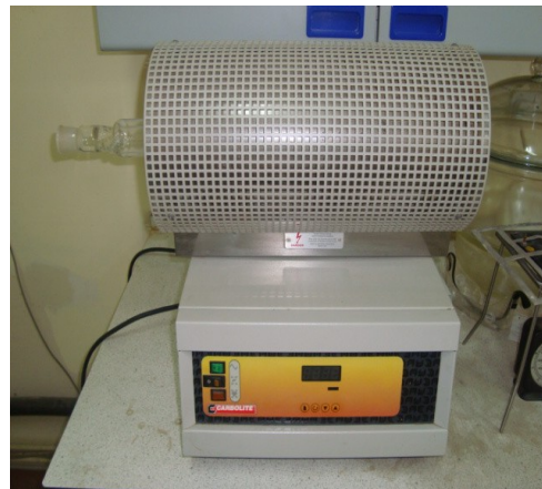
Fig3.5 a) the sputtering system used b) sputtering chamber of the system c) the carbolite furnace used for annealing.
