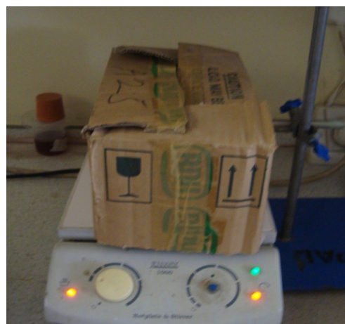
Fig 3.3 : a) the active layer being prepared on the stirrer. b) the set-up covered by a carton to minimise vaporisation.
