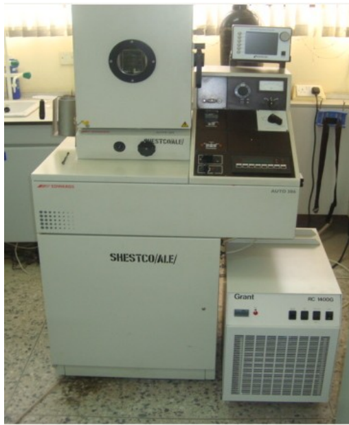
Fig 3.7a) the thermal evaporator used for the aluminium deposition. b) the evaporating chamber showing the substrate holder and filament.
