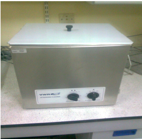
Fig 3.1: Materials used for cleaning. a) The ultrasonic cleaner. b) the nitrogen gun
