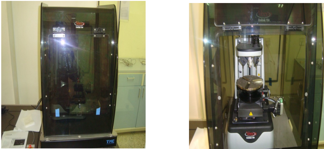
Fig 3.8: a) the Veeco surface profiler used b)the interior of the profiler
