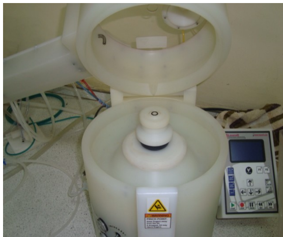
Fig 3.6: Showing the spincoating chamber and the controller*
