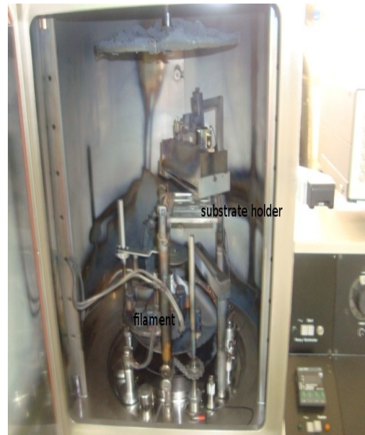
Fig 3.7a) the thermal evaporator used for the aluminium deposition. b) the evaporating chamber showing the substrate holder and filament.
