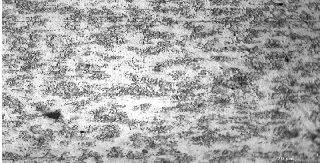
Figure 7 Microstructure of low carbon steel before exposure. 3x400
