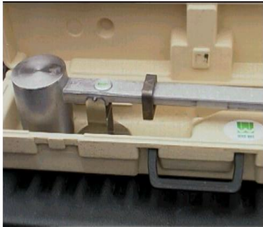
Figure 3.1: An example of a mud balance (wyo-Ben, 2011 and Bourgoyne et al., 1986).
