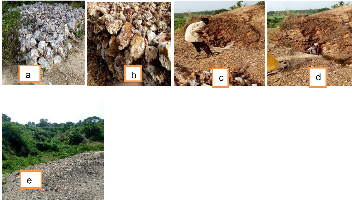
Figure 4.1: Low quality (a) and high quality (b) barite at vein 17 Azara vein 18 (c) and (d) in Azara. The vein depth is more than 30 meters.
