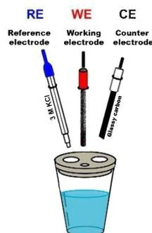
**Figure 3-2** The three-electrode cell setup
