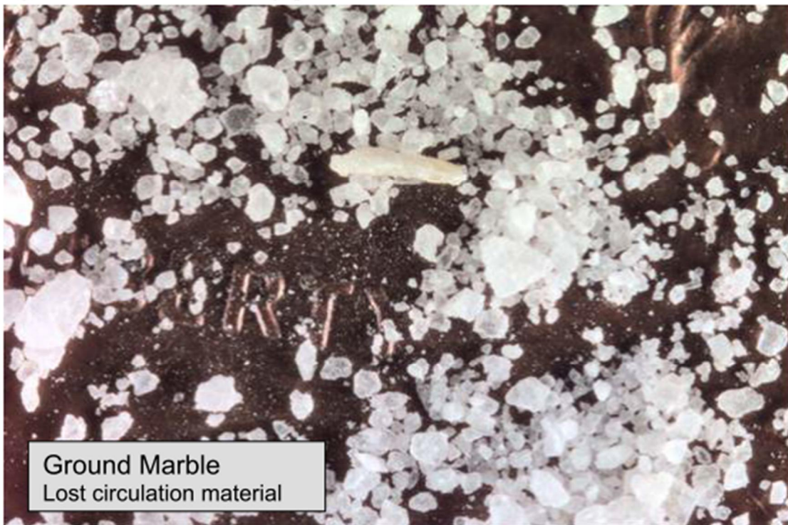
Fig. 3.2 – Particulate LCM for Wellbore Strengthening (After Wang et al. 2009).
