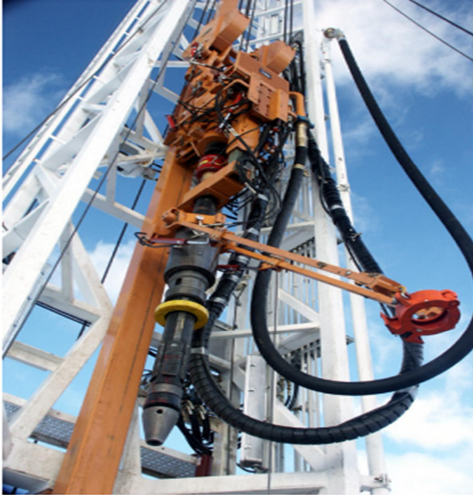
Fig. 3.3 – Top Drive and Internal Casing Drive (After Tessari et al. 2006).
