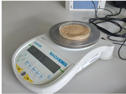
Figure 3.5: Mud Density Determination
