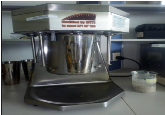
Figure 3.5: Mud Density Determination
