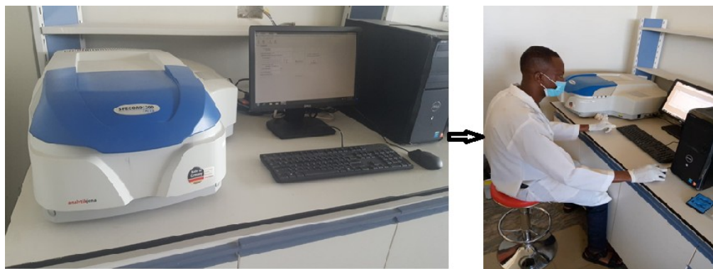
Figure 3.4: Determination of the absorption of iron oxide nanoparticles using a UV-Vis. The absorbance and concentration of iron leached were characterized using Beer-Lambert Law which follows [6] :
