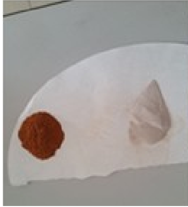
Figure 4.11: Initial Redish color of the clay sample turns to white after the leaching process.
