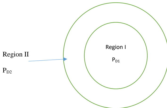
Figure 4.1: A schematic diagram of a two-region radial composite reservoir.
