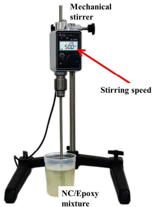
Fig. 4.2. Mechanical stirring setup for dispersion of NCs into epoxy resin
