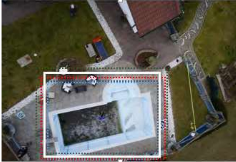
Figure 2.13: Anchor boxes (dotted) and the shift/scale applied to them to fit the object precisely (solid). Several anchors can map to the same object. Source: Author
